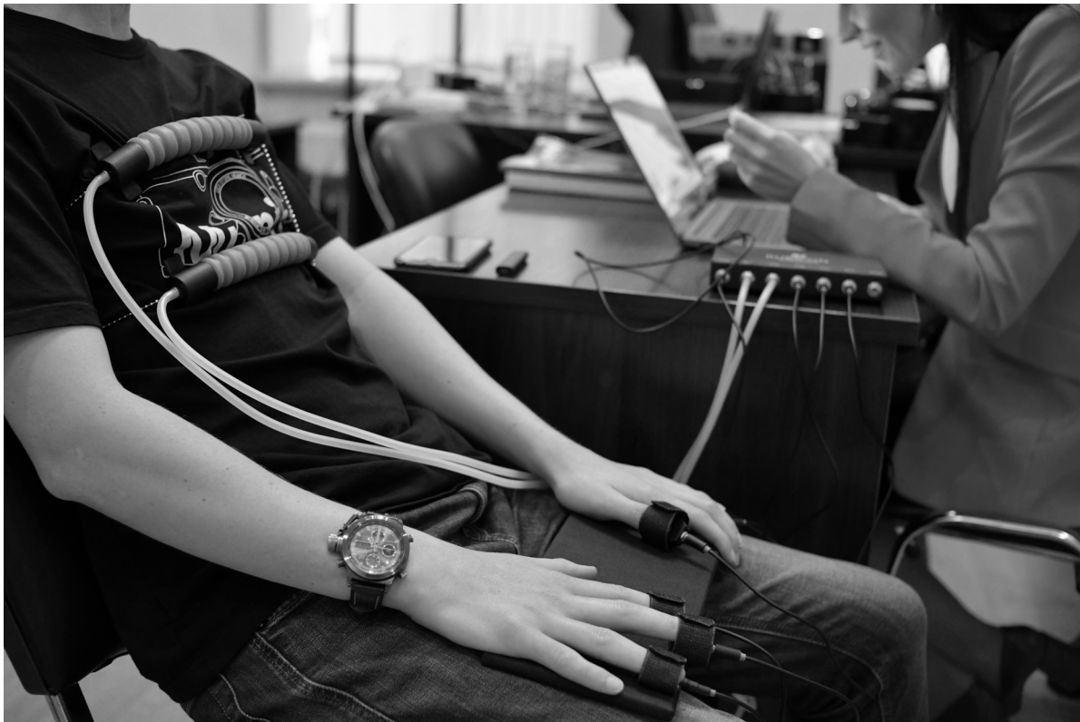
FIGURE 2. SENSORS FOR CAPTURING CUTANEOUS GALVANIC RESPONSE (CGR)
